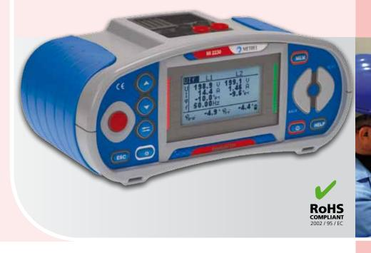
MI 2230 VAFMeter is handheld multifunction instrument which can accurately measure voltage, current, power, harmonic distortion and phase angles in single, two and three phase systems.
